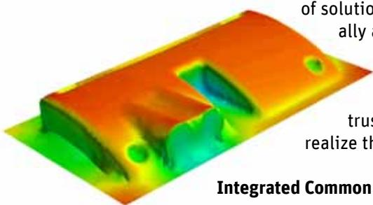
Polyflow assists in optimal thermoforming of an automotive dashboard design. Areas shown in blue are less thick, demonstrating potential design weakness.
