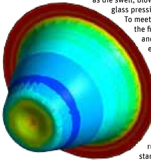
Polyflow accounts for material contact in optimizing a design, such as determining final material distribution for a plug-assist thermo-formed cup.
