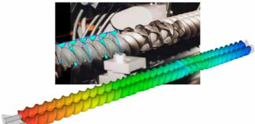
MST in Polyflow accounts for complex thermal and mechanical interactions for single- and twin-screw extruders.
